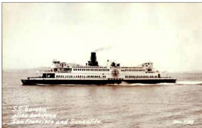
NORTHWESTERN PACIFIC’S 1890 “EUREKA”—A WALKING BEAM, DOUBLE ENDED, SIDE-WHEELER. THE STEAM POWERED FERRY HAS BEEN COMPLETELY RESTORED AND IS ON DISPLAY AT HYDE STREET PIER, PART OF SAN FRANCISCO’S MARITIME NATIONAL HISTORICAL PARK. [ZAN 1198, 1936; PRODUCTION TOTAL 10,000]
