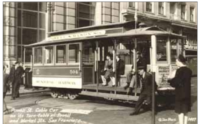
A POPULAR VIEW OF POWELL STREET CABLE CAR 504 BEING ROTATED ON THE TURNTABLE AT MARKET. THE SINGLE-ENDED CAR, BUILT IN 1887 AND MODIFIED IN 1915, CURRENTLY RESIDES ON THE UPPER LEVEL OF RIGHT-CENTER FIELD AT AT&T PARK, RENUMBERED 44 IN HONOR OF WILLIE MCCOVEY. [ZAN 2497, © NOV 8, 1946]
