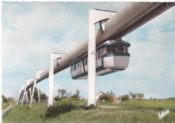
TEST TRACK OF THE SAFEGE MONORAIL NEAR PARIS
