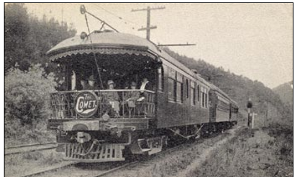
OAKLAND, ANTIOCH & EASTERN RY. car Moraga, as a double open-end observation platform, motor on train no. 2, the Comet, at Haven's Station in Shepherd Canyon about to enter the tunnel; 1914. Frank A. Jay photo.
