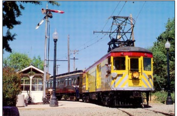
“Many electric interurban lines relied on express motors to handle less-than car load freight and as locomotives.” CENTRAL CALIFORNIA TRACTION COMPANY EXPRESS MOTOR #7—originally Washington, Baltimore & Annapolis #11, was restored in 1991 by the Western Railway Museum. “The silver stripes on the front end were intended to warn unwary motorists of its approach on Stockton and Sacramento streets.
